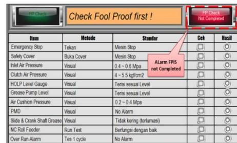
**Gambar 3.5.** Halaman HMI Check Point Not Completed
