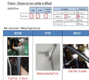
Gambar 14. Modification Tools for repairing main cylinder
