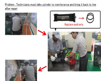
Gambar 15. Repairing main cylinder with dandory ssystem
