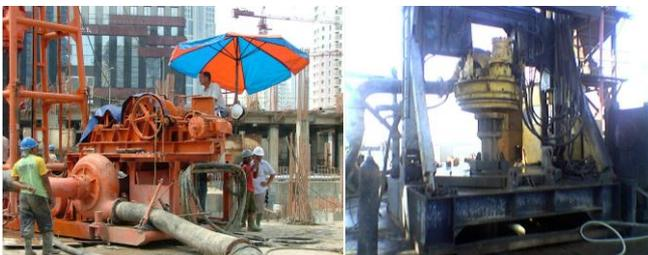
**Gambar 8. RCD Sistim Suction & Sistim airlift**
