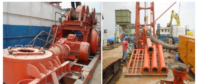
Gambar 14. Rotary Table & Heavy Duty Drilling Rod
