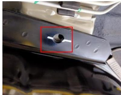
Gambar 2. Kondisi *Issue Hole Not Center* saat *install Fuel Tank*
