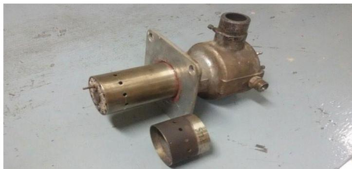
Gambar 9. perspektif burner tube (Sumber : PT EFG-Kiln Dept, 2022)
