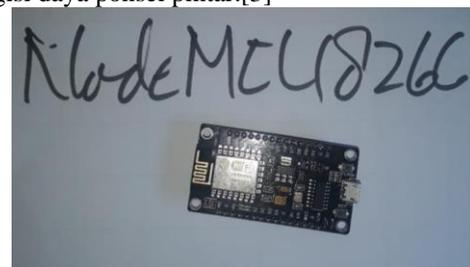
Gambar 1 NodeMCU ESP8266
