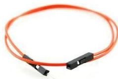
**Gambar 2.5** Kabel Jumper Male to Female
